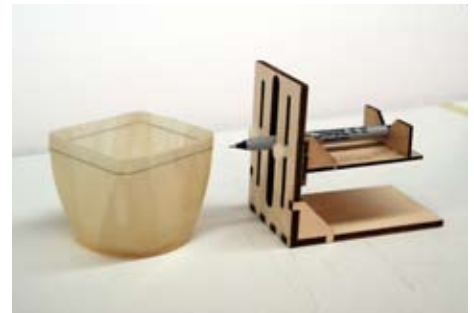
The Top Notch Height gauge is used to mark the exact location of the trim line on the fiberglass cowl. The cowl is cut to about 1/32" from this line and then sanded flat down to the line before the cowl ring is installed.
