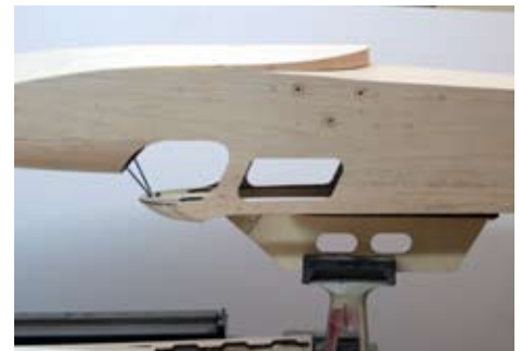
Above, the Utility handle is used to secure the fuselage assembly in preparation for glassing. This enables secure control of the fuselage without having to physically touch the fuselage assembly. This is handy for glassing and painting purposes.
