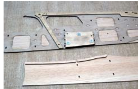
Above, the landing gear bolt plate assembly has been added with #6-32 blind nuts installed. Below, the stabilizer saddle doubler has been added.
