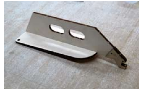
A utility handle has been provided to simplify some of the building processes. The handle mounts to the fuselage using the wing attachment system and is useful for transport as well.
