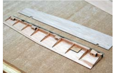
Aileron ready for the top sheeting to be installed. All ribs, hinge blocks and horn plate installed. After the top sheeting is installed the leading edge is beveled to 22° to allow for surface movement.
