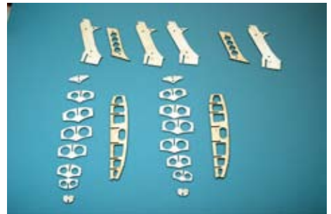
Pontoon parts ready for assembly. At the top are the pontoon pylon parts and below that the pontoon keel and formers. The built up pontoons will weigh about 1.5 ounces when finished, saving considerable weight over a solid wood carved pontoon.
