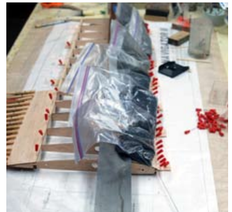
Leading edge sheeting being installed using a heavy straight edge to assure good contact between the sheeting and the spar flange. Ziplock baggies filled with lead shot conform to the airfoil and pins retain the leading edge.
