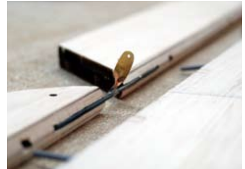
Test fitting of the elevator torque rod in the elevator halves. This will be permanently installed after covering or finishing. The forward rake of the horn is offset by an equivalent offset on the servo arm for equal throws.
