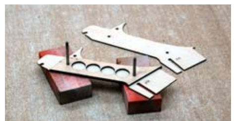
Pylons are assembled using the pin registration method.
