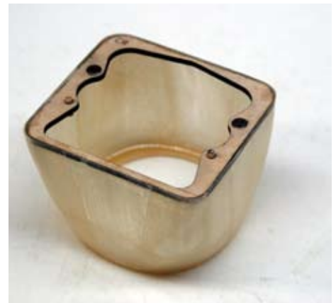
The completed cowl assembly. The two 1/8" alignment dowels and four magnets provide a perfectly aligned and firm mount to the power pod. This method allows quick access to the motor as well as eliminates the need for unsightly retaining screws.
