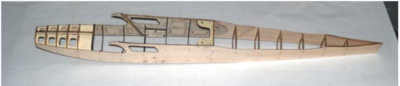
The fuselage assembly underway with the nose section subassembly and all formers installed as well as the wing bolt plate. Note that the fuselage sides will stand slightly proud of the former tabs to allow easier filling and sanding of the finished sides.
