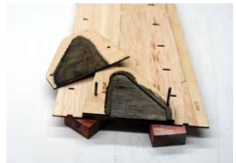
The aluminum sponson mount pocket must be waterproofed with Epoxy resin. Here the resin has been tinted to show where this needs to be done. Do not omit this step.
