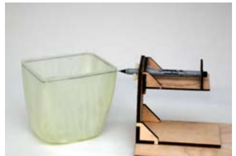
The Top Notch Height gauge is used to mark the cowl exactly 4-3/8" back from the spinner ring. The cowl is then trimmed about 1/32" shy of this line and then sanded flat back to this line.
