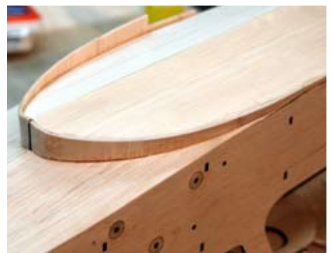
Sheeting of the step underway here. The step sheeting is sanded flat on the sides to fair in with the fuselage sides.
