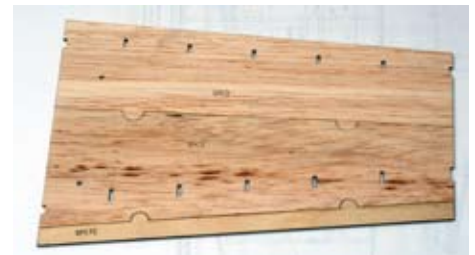
The sponson core sheet assembly ready for assembly.
