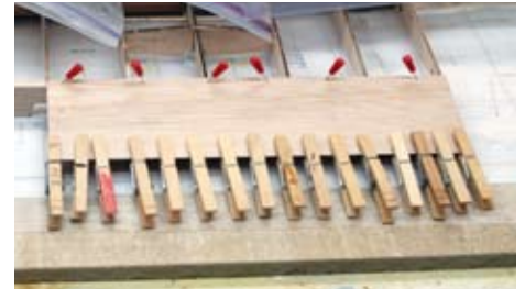
Wing sheeting panel H is installed using pins along FTE and lots of clothes pins along the trailing edge to assure a good bond along the trailing edge.
