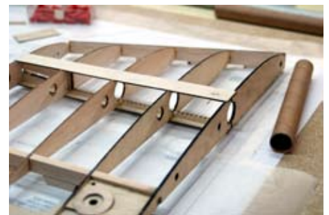
All the dash cut material has been removed from the sheer webs and the ribs in preparation for the installation of the wing tube sleeve. The sleeve will now be installed and secured with a liberal application of Aliphatic Resin glue at all contact points with the wing. Note also that WBT has been installed on WBP and planed to contour with the ribs in preparation for sheeting.
