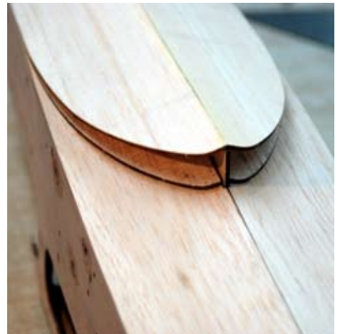
FSP and the forward bottom sheeting define the step outline shown here. All that remains is to create this neat step is to sheet these elements.
