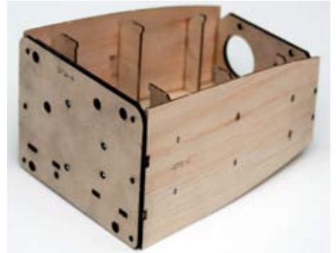
Basic glow power pod structure ready for corner bracing and sheeting. Throttle servo and tank are also mounted in the pod.
