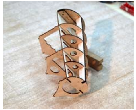
This nose section subassembly will force the fuselage sides into perfect alignment when installed and eliminate any chance of building a banana.
