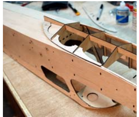
Sheeting begins with the aft bottom sheeting and FSP is then installed over this. FSP will provide the top of the step sheeting a ledge to glue to. The bottom of the step sheeting support will be the forward bottom sheeting.
