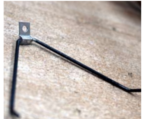
The cabin brace as supplied is fabricated from 3/32" music wire and a steel cable clip silver soldered together. The brace is a structural element and must be installed as indicated with the supplied hardware. After installation secure all contact points with thick CA or Epoxy.
