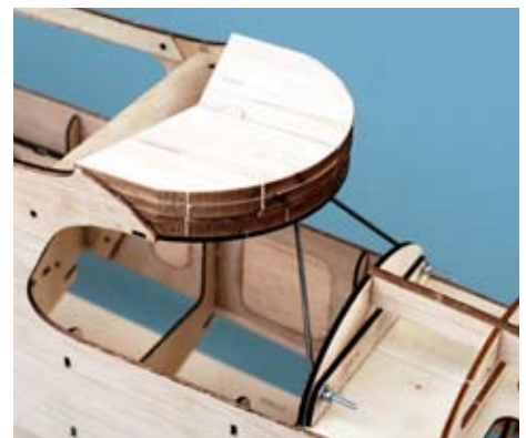
The cabin roof is built up of laminations of balsa after installing the cabin brace and bolting in place. The ply plate at the bottom of this structure also holds the hardwood forward wing attach dowel.
