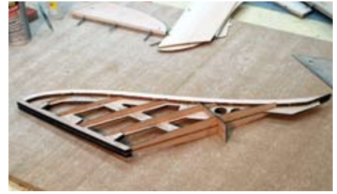
Vertical fin assembly ready for laser cut sheeting. The tab at the front engages the top keel and V5 will glue to former F15 for a solid aligned installation.
