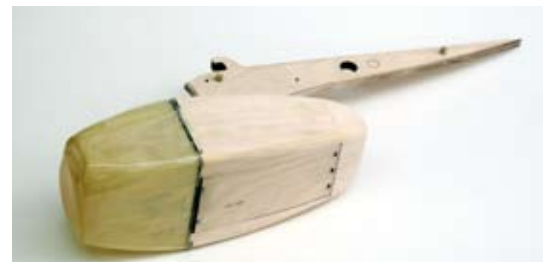
The completed glow power pod will hold a 12 oz. tank and the throttle servo. The throttle servo is accessible by a small hatch on the bottom. The top hatch is retained by two dowels and two screws. The radio switch can also be installed in the power pod.
