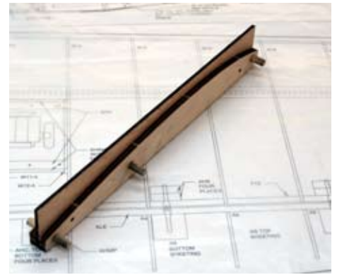
The assembled W1 FIXTURE is used to assure that rib W1 retains its correct shape while the assembly is being done. W1 must interface with the pylon and must retain the same profile.
