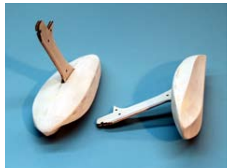
The finished pontoon and pylon assemblies ready to be glassed. The pylons are not attached to the pontoons until after glassing and then a small fillet is formed along the pylon and pontoon.
