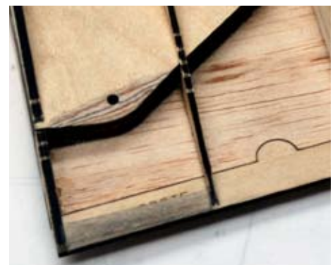
A piece of scrap balsa has been installed between SP1-B and SP2-B and tapered to contour. Above this, the SPSS assembly has been tapered to clear the 3/32" bottom sheeting.
