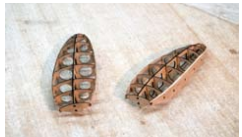
Assembly underway, the pontoons are ready for the top and bottom sheeting. The top and bottom 1/16" sheeting will be installed wet for bending.
